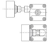
The switch is provided with a wide centering inlet for the actuator pin. Such solution makes it easier to align the actuator with the hole found in the head during the fitting stage. Moreover, this solution drastically reduces any probable collisions between the actuator and the switch, also allowing it to be fitted on inaccurate doors.
