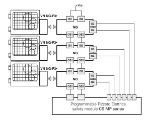
Possible connection in series of several switches in order to simplify the safety system wiring, after evaluating the outputs from the last switch in the chain by means of a safety module from Pizzato Elettrica CS MP series, which allows management of both safety and signalling
