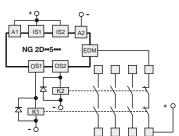
The NG 2D••5••• version, in addition to maintaining the operating and safety characteristics of the NG series, allows control of forcibly guided NC contacts of contactors or relays controlled by the safety outputs of the switch itself. As an alternative to the relays or con-
