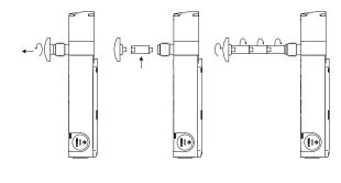
Metal extensions can be combined together until the required length is obtained. Do not exceed an overall length of 500 mm between the release button and the
