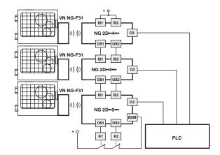
This version, with the IS safety inputs, can be used at the end of a series of NG switches, up to a maximum number of 32 devices, while maintaining the maximum PL e safety level and acc. to EN ISO 13849-1 and SIL 3 safety level acc. to EN 62061.
