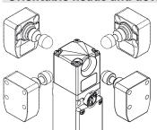
The head can be quickly oriented in four different directions after unscrewing the 4 fixing screws. Also the key release device and the emergency release button can be positioned in 90° steps, thus obtaining as many as 16 different configurations with the same article.
