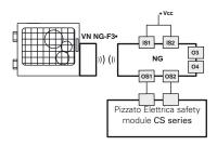
The NG series switch can be used individually, prior evaluation of the safe outputs by means of a Pizzato Elettrica safety module (see table for safety modules to be combined).
