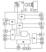
The diagram on the side represents the 6 logic functions which interact inside the device.
