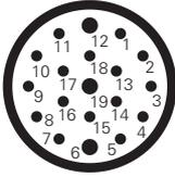
To connect the switch contact block to the 19-pole M23 connector, see pin numbers 1 to 10 of the diagrams on page 17.
