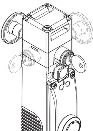
The key release device (auxiliary release) is used to permit unlocking of the actuator only by personnel in possession of the key. The device also functions with no power supply and, once actuated, prevents the guard from being locked.
