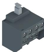
Innovative contact block with 4 contacts, available in various contact configurations for monitoring the actuator or the solenoid (patented). The unit is supplied with captive screws and self-lifting clamping plates. Removable finger protection for eyelet terminal.
