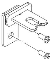
As required by EN ISO 14119, the actuator must be fixed immovably to the guard frame. Pan head safety screws with one-way fitting are available for this purpose. With this screw type, the actuators cannot be removed or tampered by using common tools. See accessories on page 359 of the General Catalogue Safety 2021-2022.
