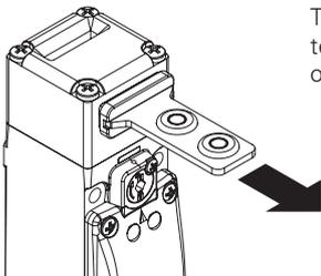
The strong interlocking system guarantees a maximum actuator holding force of  $F_{1max} = 2800 \text{ N}$ .
