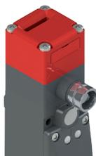
Articles with the V70 and V73 option have an auxiliary key release with a triangular key that meets DIN 22417 standards. This type of lock can be used in situations where the switch must only be unlocked using the corresponding triangular key, a tool which is not usually available. There are two versions of the triangular key release: with a spring return (option V70) and without a spring return (option V73).
