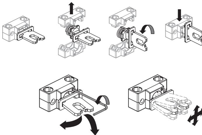
Jointed actuator for guards with poor alignment, adjustable in two dimensions for small doors; can be mounted in various positions. The metal fixing body has two pairs of bore holes; it is provided for rotating the working plane of the actuator by 90°.
