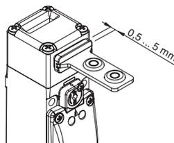
The actuation head of this switch features a wide range of travel. In this way the guard can oscillate along the direction of insertion (4.5 mm) without causing unwanted machine shutdowns. This wide range of travel is available in all actuators in order to ensure maximum device reliability.
